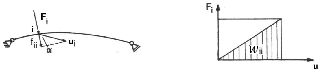
Fig. 41. Force \mathbf{F}_i , acting at point i of a beam, causing the displacement (projection) f_{ii} in the direction of \mathbf{F}_i .
