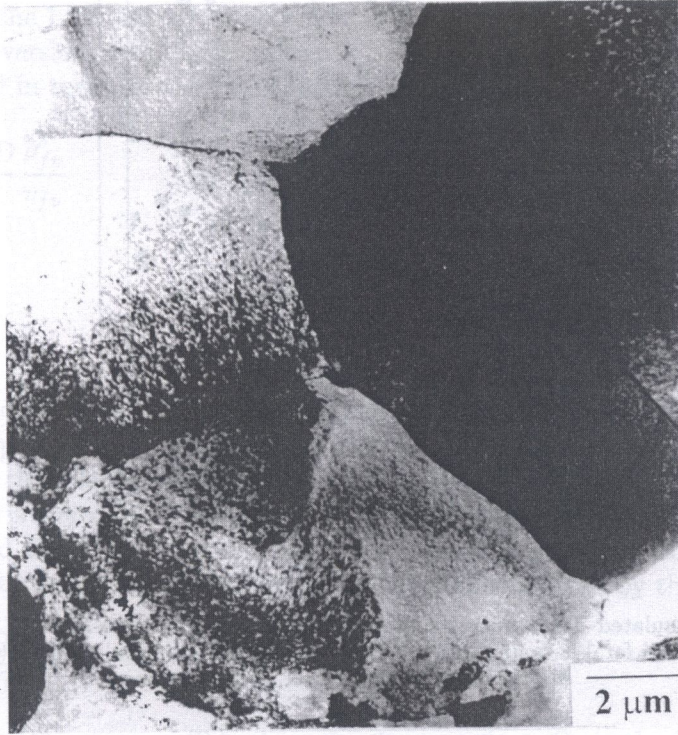
Fig. 3. Dark field TEM micrograph showing the dislocation subgrain structure of the Al-2.6wt.% Li 0.09wt.% Zr Alloy in the peak-aged condition, artificially aged at 185° C for 48 hours, (12000X), from TEM thin foil specimens
