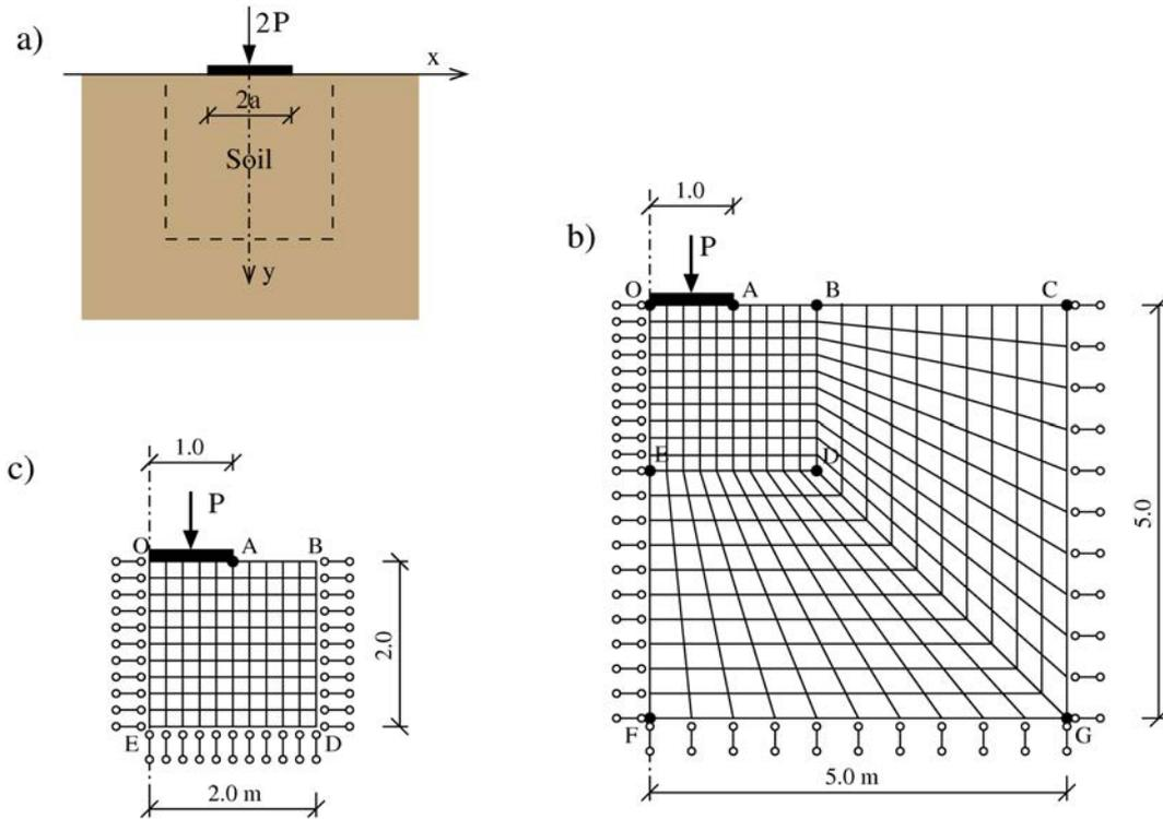
Fig. 2. Plane strain BV problems discussed: a) infinite semi-space, b) finite domain O-C-G-F, c) finite domain O-B-D-E.
