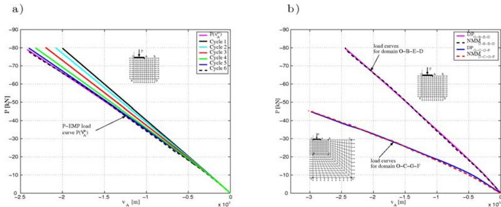
**Fig. 3.** a) Equilibrium paths  $P(v_A)$  computed for O-B-D-E domain during training  $\text{NMM}_{\text{O-B-D-E}}$  process; b) pseudo-empirical equilibrium paths  $P(v_A)$  computed by FEM/DP and FEM/ $\text{NMM}_{\text{O-B-D-E}}$  program.
