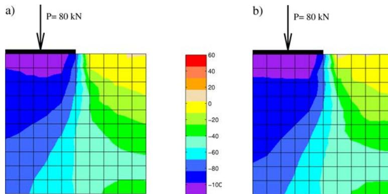
Fig. 4. Distribution of  $\sigma_{pde}(x, y)$  for O-B-D-E domain for a) equivalent NMM<sub>O-B-D-E</sub> model, b) DP model.
