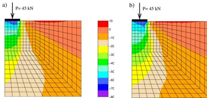
Fig. 5. Distribution of  $\sigma_{pde}(x, y)$  for O-C-G-F domain for a) equivalent NMM<sub>O-B-D-E</sub> model, b) DP model.
