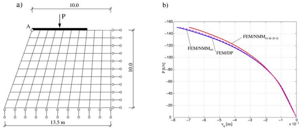
**Fig. 6.** a) Geometry of slope; b) equilibrium paths  $P(v_A)$  computed by FEM/DP, FEM/NMM<sub>O-B-D-E</sub> and FEM/NMM<sub>ret</sub> hybrid program.
