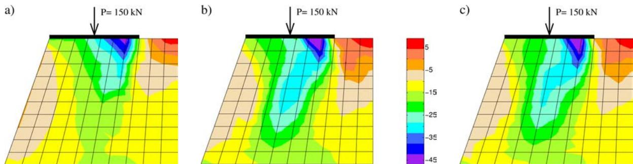
**Fig. 7.** Distribution of  $\sigma_{pde}(x, y)$  for: a) equivalent NMM<sub>O-B-D-E</sub> model, b) equivalent NMM<sub>ret</sub> model, c) DP model.
