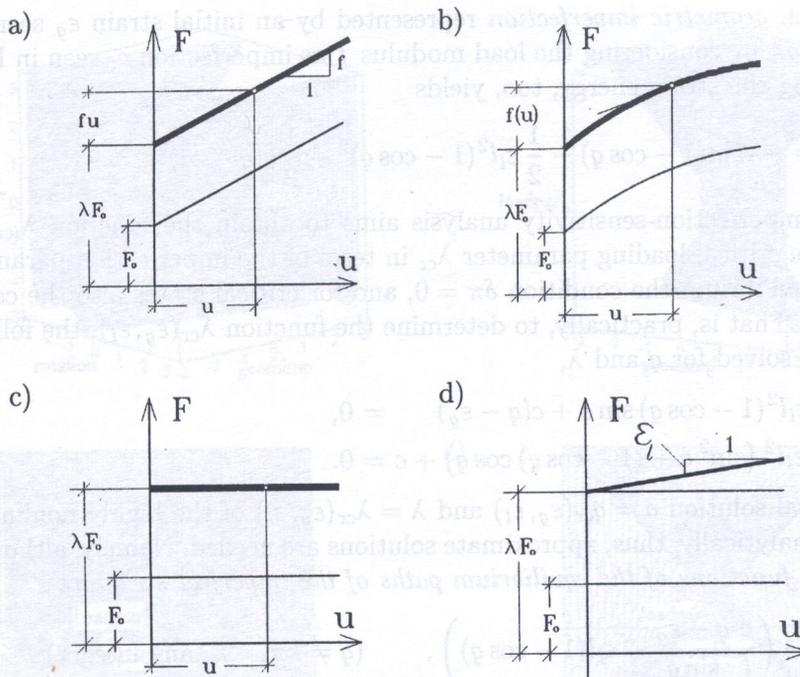
Fig. 2. The configuration-dependent loading and the loading imperfection; a) linear configuration-dependent loading, b) nonlinear configuration-dependent loading, c) dead loading, d) loading imperfection
