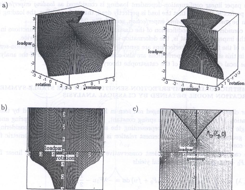
Fig. 3. Geometric imperfection-sensitivity; a) equilibrium surface  $\lambda(q, \epsilon_g, 0)$ , b) sections of  $\lambda(q, \epsilon_g, 0)$  for constant  $\epsilon_g$ , c) section  $\lambda_{cr}(\epsilon_g, 0)$  of the imperfection-sensitivity surface  $\lambda_{cr}(\epsilon_g, \epsilon_l)$
