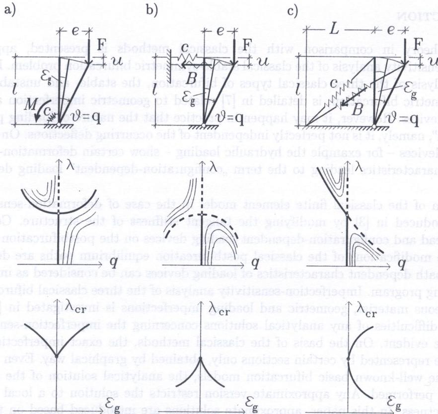
Fig. 1. The three classical bifurcation models, equilibrium paths and the classical imperfection-sensitivity functions; a) stable-symmetric, b) unstable-symmetric, c) asymmetric
