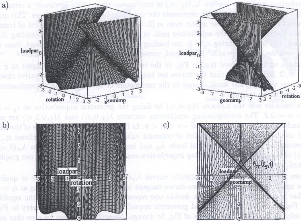
Fig. 4. Geometric imperfection-sensitivity influenced by loading imperfection; a) equilibrium surface  $\lambda(q, \epsilon_g, 1)$ , b) sections of  $\lambda(q, \epsilon_g, 1)$  for constant  $\epsilon_g$ , c) section  $\lambda_{cr}(\epsilon_g, 1)$  of the imperfection-sensitivity surface  $\lambda_{cr}(\epsilon_g, \epsilon_l)$
