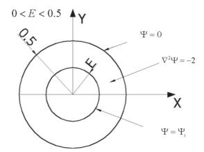
Fig. 4. Formulation of boundary value problem for circular with circular centered hole cross section of a bar. Problem I.
