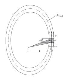
Fig. 3. Thin-walled bar with closed cross-section.
