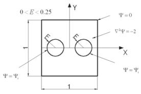
Fig. 8. Formulation of boundary value problem for square with two circular symmetrically placed holes section of a bar. Problem V.
