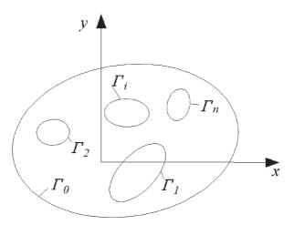
Fig. 1. Multiply connected cross sections of bar.
