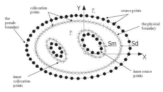
Fig. 2. Arrangement of the source points on the similar contour.
