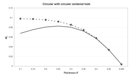
Fig. 10. Comparison of results given by proposed formula (19) – points, Bredt's formula (23) – solid line and exact solution (22) – broken line for circular with circular centered hole; M = 46, NC = 46.
