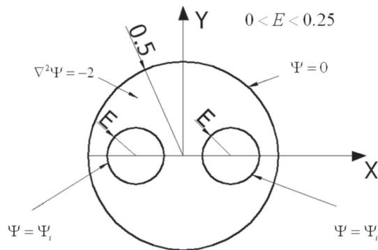
Fig. 7. Formulation of boundary value problem for circular with two circular symmetrically placed holes cross section of a bar. Problem IV.
