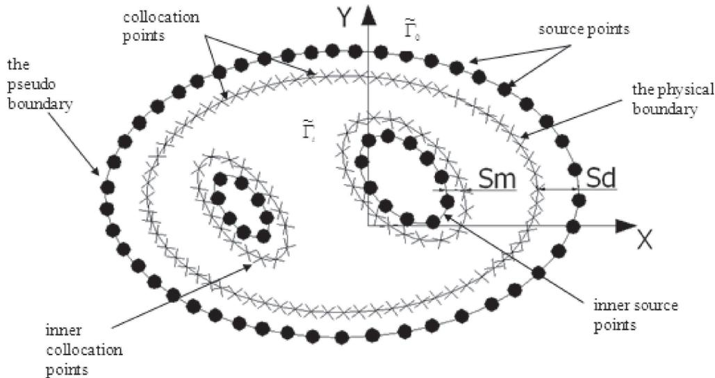
Fig. 2. Arrangement of the source points on the similar contour.
