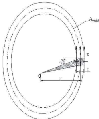
**Fig. 3.** Thin-walled bar with closed cross-section.
