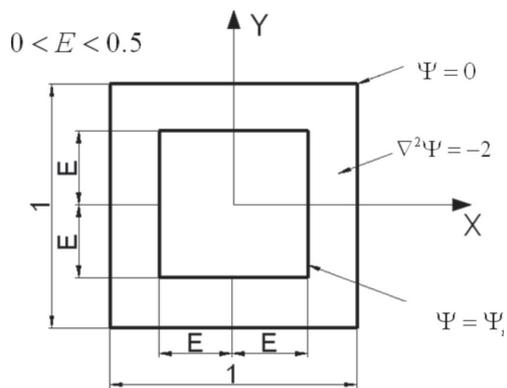
Fig. 6. Formulation of boundary value problem for square with square centered hole cross section of a bar. Problem III.
