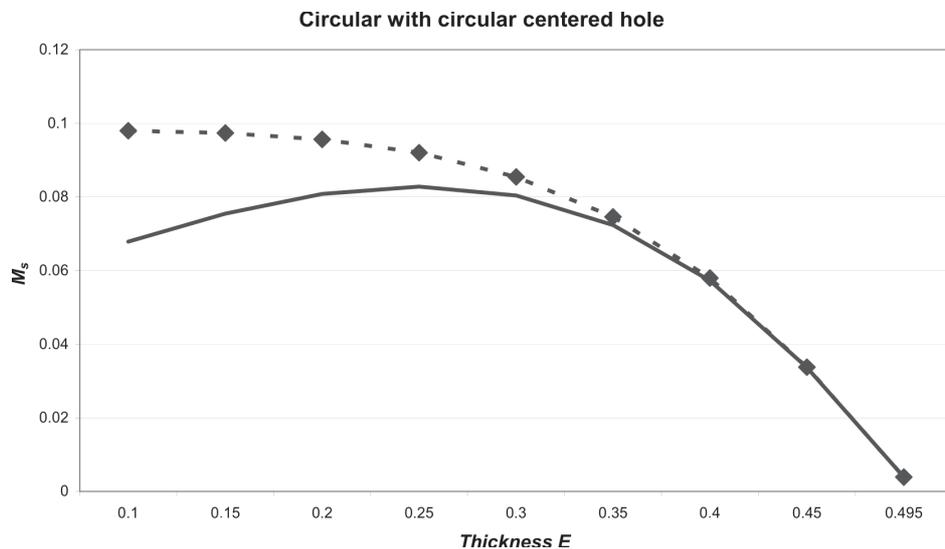
**Fig. 10.** Comparison of results given by proposed formula (19) – points, Brecht's formula (23) – solid line and exact solution (22) – broken line for circular with circular centered hole;  $M = 46$ ,  $NC = 46$ .
