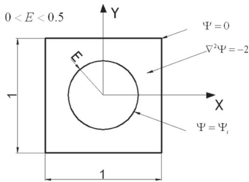
Fig. 5. Formulation of boundary value problem for square with circular centered hole cross section of a bar. Problem II.
