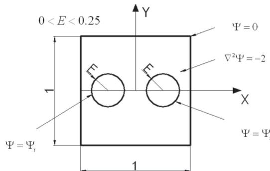
Fig. 8. Formulation of boundary value problem for square with two circular symmetrically placed holes section of a bar. Problem V.
