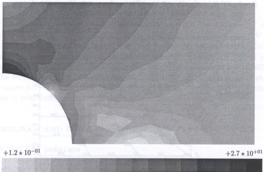
Fig. 7. Distribution of equivalent stress \sigma_e zones for \chi = 0.032 and u_A = 0.55 mm
