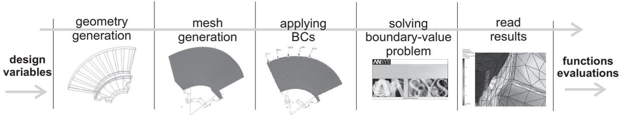
Fig. 3. Steps in calculation of the fitness functions
