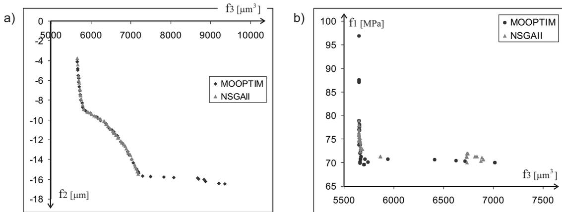
Fig. 5. Pareto-optimal solutions for the electrothermal actuator: (a) volume minimization (10) and deflection maximization (9), (b) volume minimization (10) and equivalent stress minimization (8)
