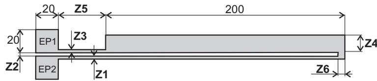
Fig. 4. Geometry and design variables of the thermal actuator
