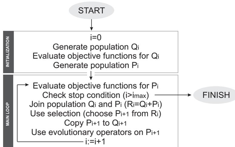
Fig. 1. The flowchart of the multiobjective evolutionary algorithm MOOPTIM
