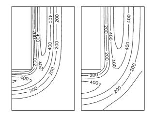
Fig. 7. Distribution of function  $\partial T/\partial c_{\rm m}$  for times 30 and 90 s
