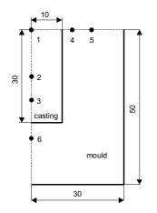
Fig. 9. Position of sensors
