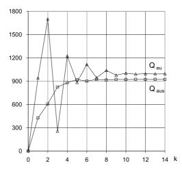
Fig. 13. Identification of  $Q_{aus}$  and  $Q_{eu}$  (optimal sensors C, D, E – Fig. 8)
