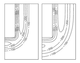
**Fig. 6.** Distribution of function  $\partial T/\partial \lambda_{\rm m}$  for times 30 and 90 s
