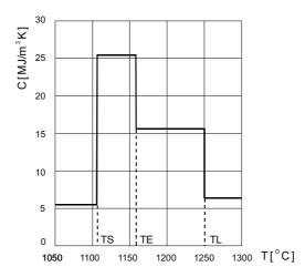
Fig. 1. Substitute thermal capacity of cast iron
