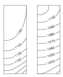
Fig. 4. Temperature distribution in casting subdomain
