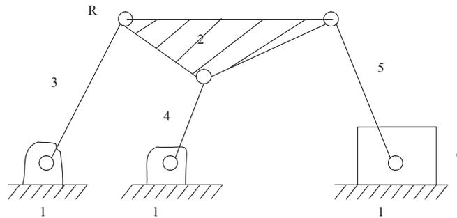
**Fig. 5.** Six-bars slider crank mechanism
