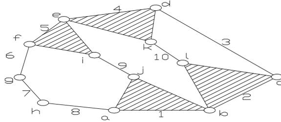
**Fig. 3.** Ten-links three-degrees-of-freedom kinematic chain
