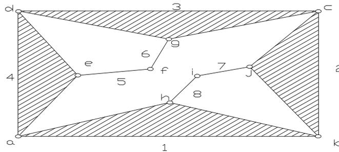
**Fig. 1.** Eight-links single-degree-of-freedom kinematic chain
