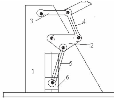
Fig. 6. Six bar slider crank mechanism
