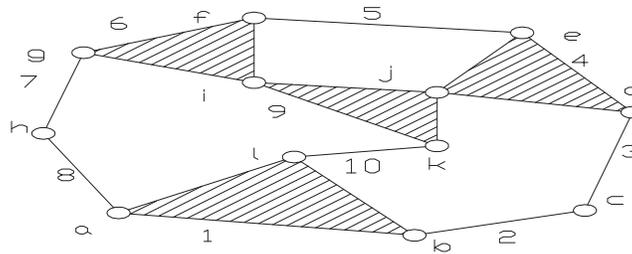
**Fig. 4.** Ten-links three-degrees-of-freedom kinematic chain
