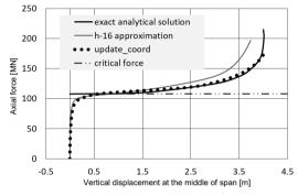
FIG. 5. Post-buckling behavior of the numerical solution for different approaches.
