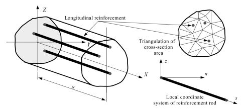
FIG. 2. Spatial frame finite element.
