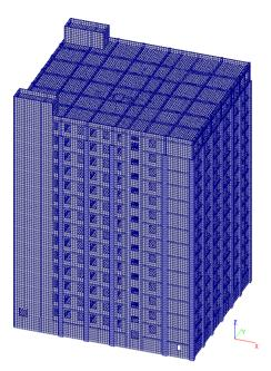
FIG. 10. Design model of a multi-story building (1027082 equations).
