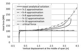
FIG. 4. Post-buckling behavior of the numerical solution while holding a different number of series terms in the Taylor expansion.
