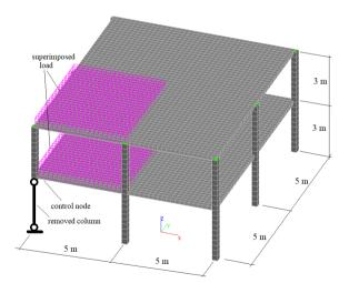
FIG. 7. Design model of the experimental sample.
