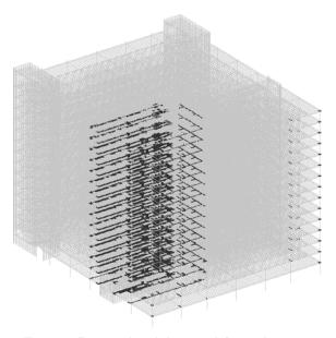
FIG. 15. Damaged and destroyed finite elements.
