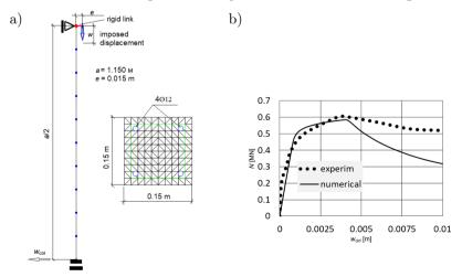
FIG. 6. a) Design model, b) longitudinal force in the bottom finite element versus control displacement.
