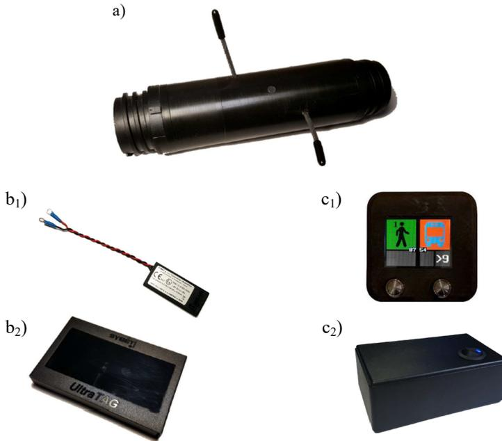
FIG. 1. Devices used in the CAS that was utilized in the studied mine: a) gate for data transmission, b) passive units ( $b_1$  – mounted in workers' mining lamps,  $b_2$  – mounted at other locations), c) active units ( $c_1$  – display for the machine operator,  $c_2$  – active device mounted on machines).
