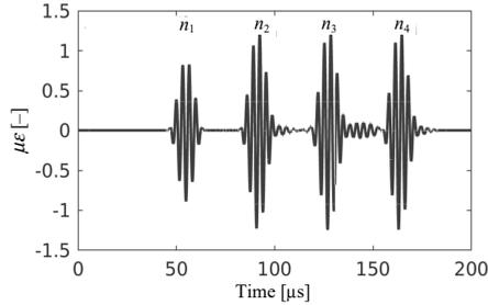
FIG. 3. Simulated time signal for healthy condition.
