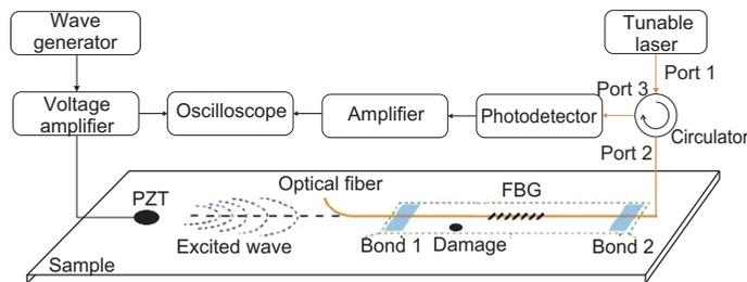
FIG. 1. Schematic explaining self-referencing configuration (based on [22]).
