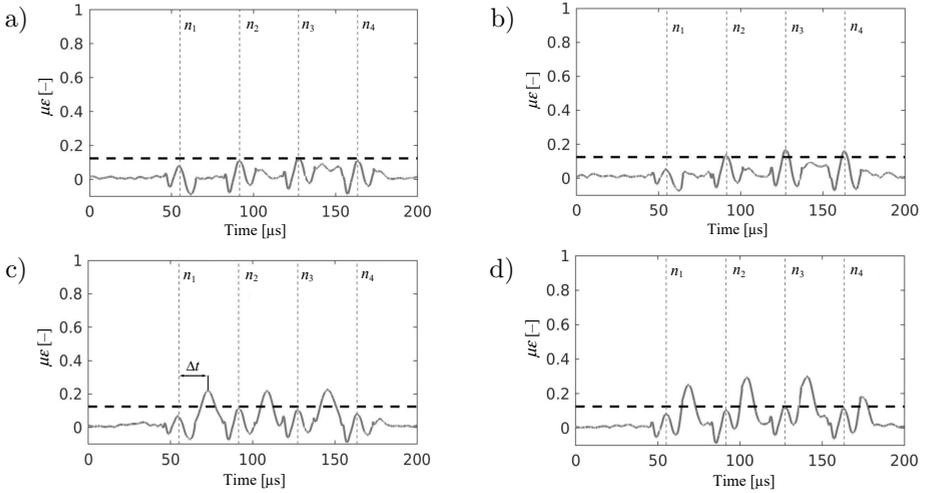
FIG. 5. Residual signal after baseline subtraction: a) healthy, b) case D5, c) case D3, d) case D4.
