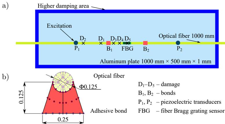
FIG. 2. Structural model (a) top view of the sample, (b) cross-section of the optical fiber and adhesive bond.
