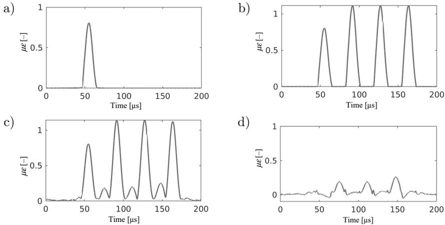
FIG. 4. Methodology for ToA-based damage localization: a) first package, b) analytical baseline signal (amped up & duplicated), c) measured signal, d) residual signal (subtraction).
