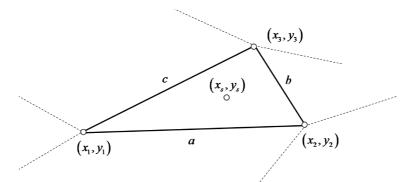
Fig. 9. Geometry of a Delaunay triangle.
