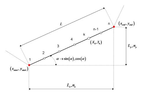
Fig. 4. Generation of nodes on the straight boundary line.
