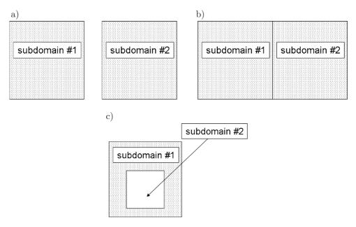
Fig. 1. Different types of 2D geometry modelling: a) two separate subdomains, b) two adjacent subdomains (one common side), c) domain with a hole.
