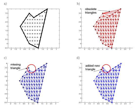
Fig. 11. Example of mesh completion with missing triangle: a) the domain and the cloud of nodes, b) direct result obtained from the "delaunay" function, c) result after the elimination of obsolete triangles, d) result after the mesh completion.
