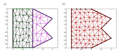
**Fig. 12.** Examples of non-conforming meshes and one consistent mesh: a) example #1 – two independent meshes, b) example #2 – one consistent mesh.
