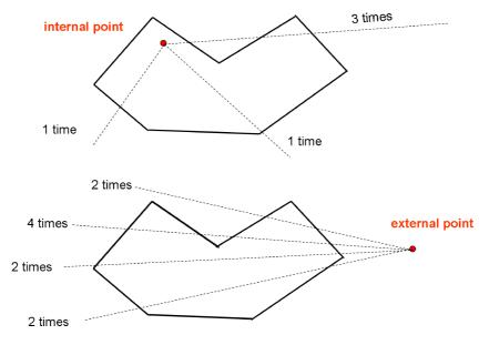
Fig. 6. Illustration for the ray-casting algorithm.
