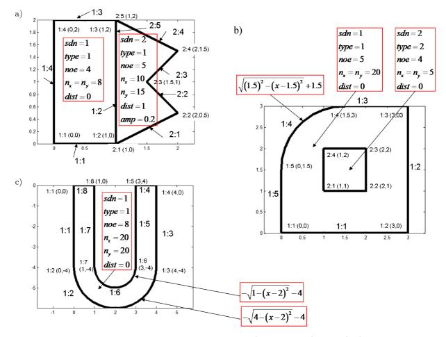
Fig. 2. Geometry data for three benchmark examples: a) example #1 (data = 1), b) example #2 (data = 2), c) example #3 (data = 3).
