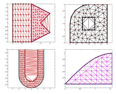
Fig. 8. Examples of Delaunay tessellation in Matlab – direct application of *delaunay* function.
