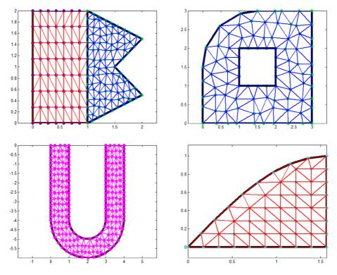
Fig. 10. Examples of proper triangular meshes.
