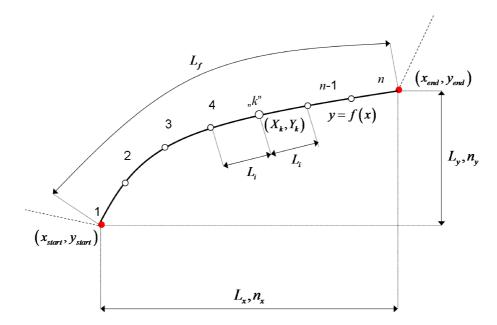
Fig. 5. Generation of nodes on the curved boundary line.
