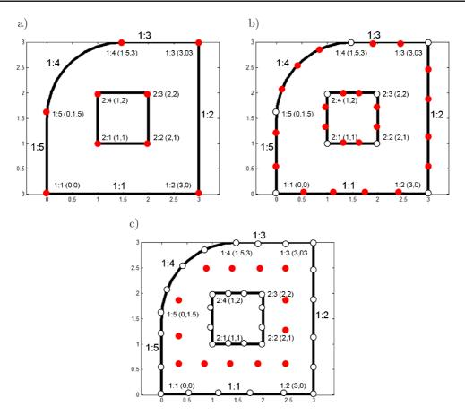
Fig. 3. Illustration of the three steps for cloud of nodes generation technique (black dots indicate new nodes for each step): a) example #2 – nodes at vertices, b) example #2 – nodes along the edge lines-curves, c) example #2 – internal nodes.
