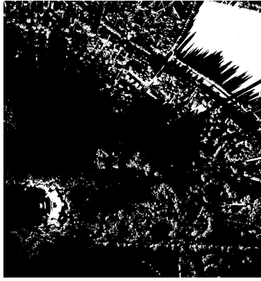
(a) Viewshed diagram generated with a 30 cm minimum point spacing
