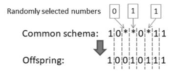
Fig. 2. Example of offspring generated from common schema. Offspring '10010111' is generated from the common schema '10\*\*0\*11'.
