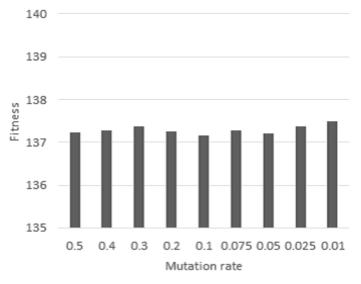
Fig. 6. Effect of mutation rate on average values of the best individuals at the final step in GE-SSE. The figure is plotted with the mutation rate as the horizontal axis and the average value of the best individuals' fitness, respectively.
