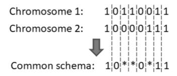
Fig. 1. Example of bitstrings and common schema. The common schema 10\*\*0\*11 is extracted from two individuals 10110011 and 10000111.
