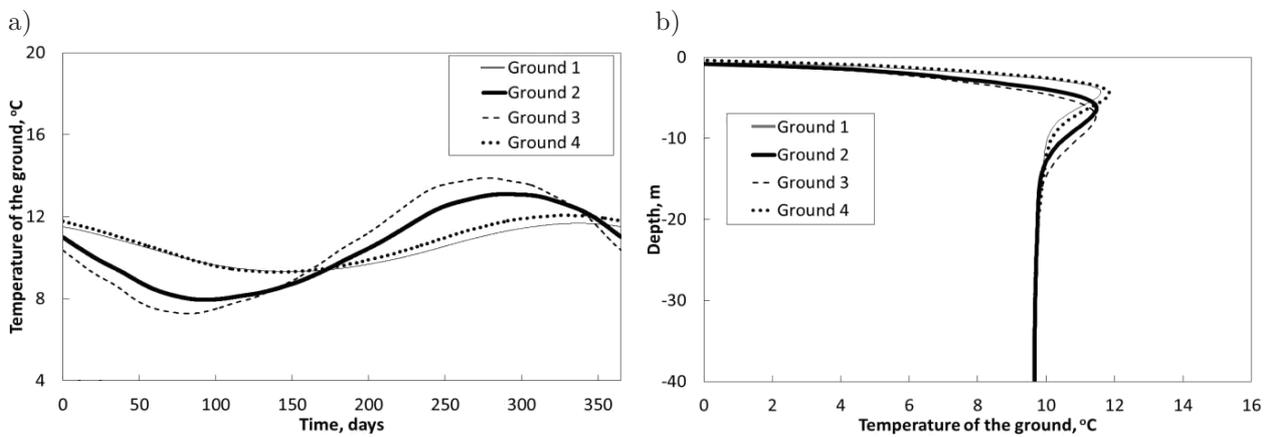
**Fig. 6.** Temperature of the ground calculated with Model 5 for different ground types for  $x = 15$  m,  $y = 15$  m: a) at  $z = 5$  m and b) profile of temperature on the end of simulation.
