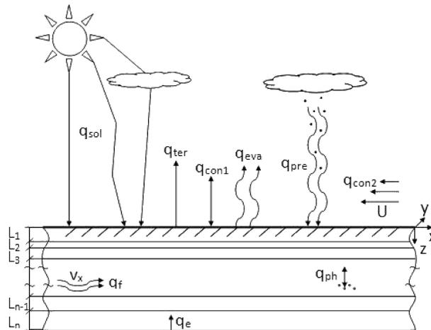
Fig. 1. Main elements of energy balance on the top surface and in the ground.
