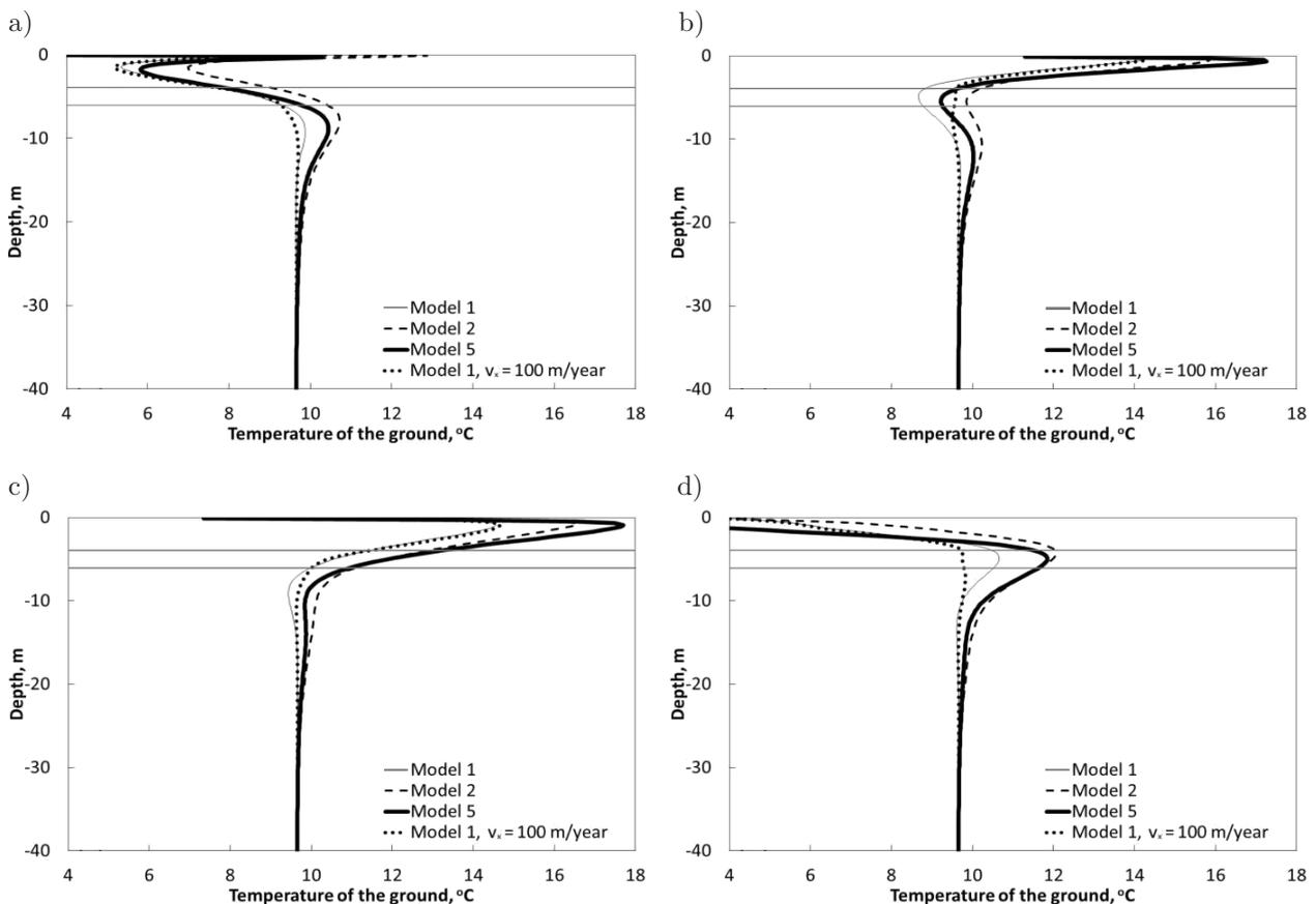
Fig. 4. Temperature of the ground type 2 for months: a) March, b) June, c) September and d) December.
