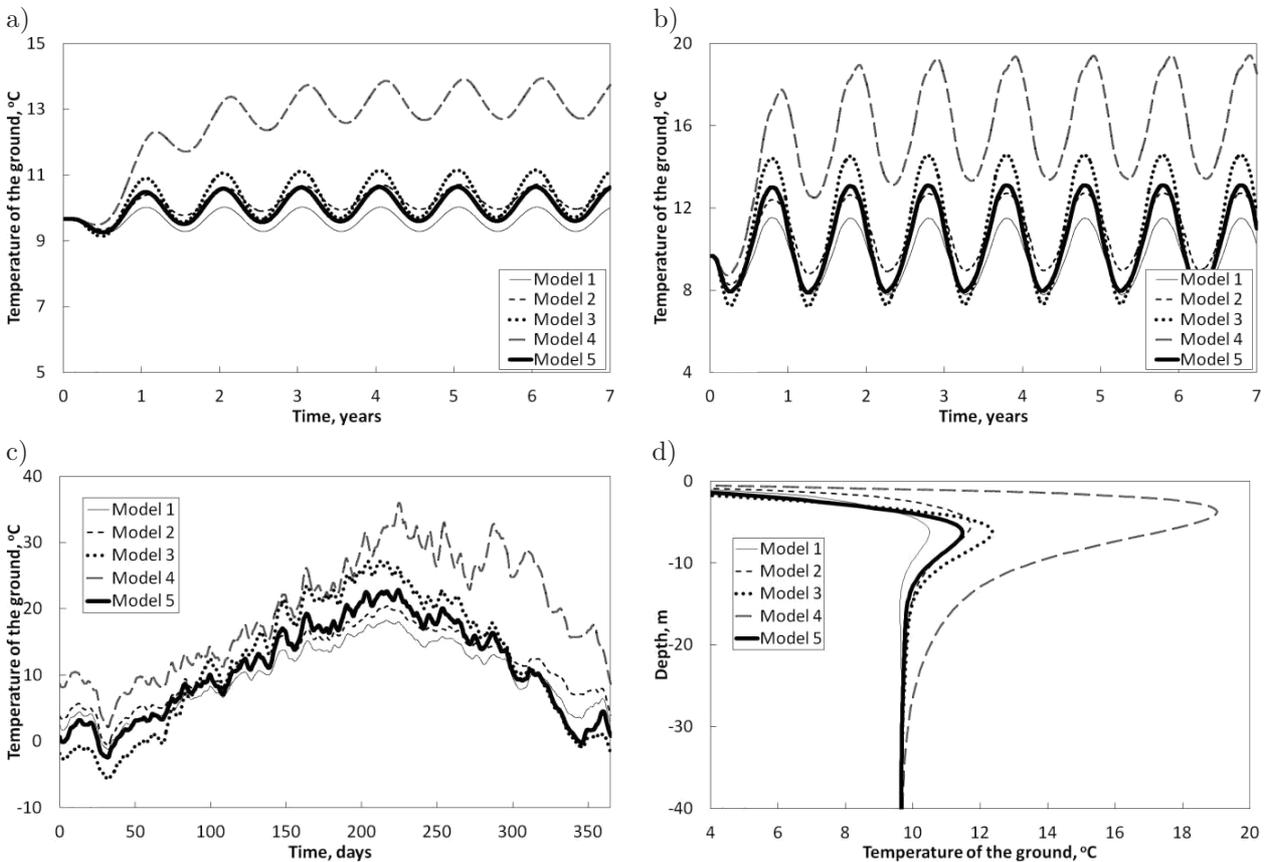
**Fig. 3.** Comparison of models for ground type 2 for  $x = 15$  m,  $y = 15$  m and at depth: a)  $z = 10$  m, b)  $z = 5$  m, and c)  $z = 1$  m, and d) temperature profile at the end of simulation.
