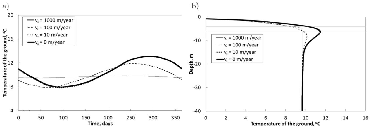
**Fig. 5.** Temperature of the ground type 2 for Model 5 for various groundwater flow speeds for  $x = 15$  m,  $y = 15$  m: a) at  $z = 5$  m and b) profile of temperature at the end of simulation.
