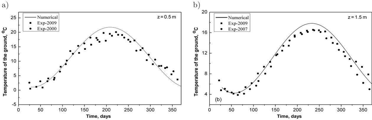
**Fig. 2.** Calculated temperature vs experimental measurement for region of Poznań City [16] and depth: a)  $z = 0.5$  m and b)  $z = 1.5$  m.
