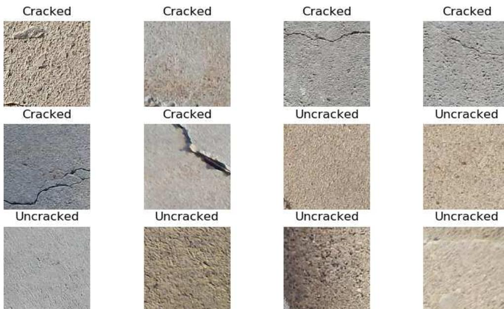
Fig. 3. Images of cracked and uncracked concrete pavements, sampled from SDNET2018 dataset.
