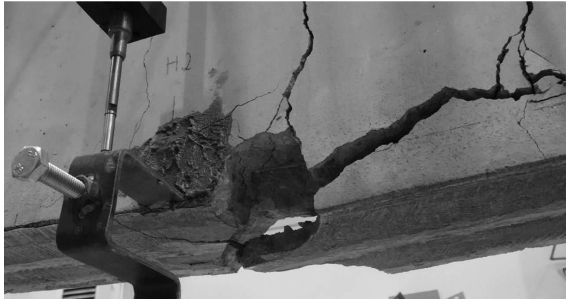
Fig. 5. Rupture of the composite material.
