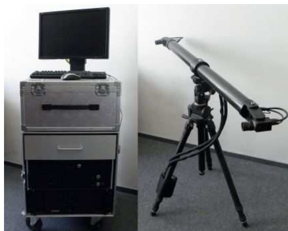
Fig. 4. Aramis system (digital image correlation).
