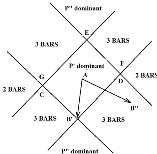
FIG. 5. Truss type as a function of the alternative loading.
