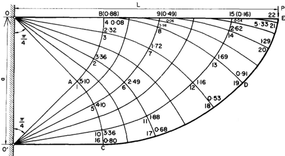
Fig. 4b. The optimal solution of a cantilever disk loaded by a concentrated force.
