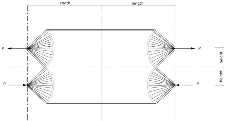
Fig. 2a. Cox's optimal beam for bending.
