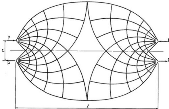
Fig. 2b. The optimal solution for pure bending presented by Chan [67].
