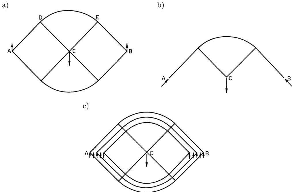
FIG. 3. Examples of non-uniqueness by Shield: a) sliding support direction, b) hinge support, c) distributed sliding support.
