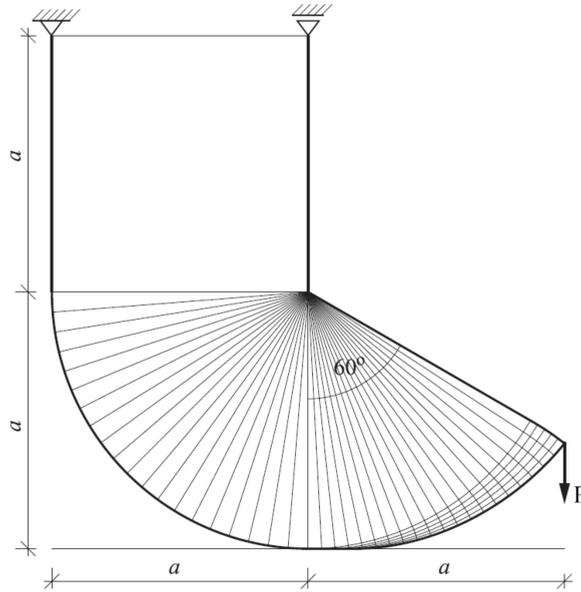
FIG. 7. The exact optimal solution of the L-shape beam by Lewiński and Rozvany [133].
