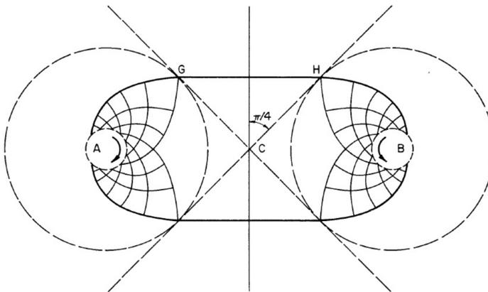
Fig. 2c. The optimal solution for pure bending presented by Shield [72].
