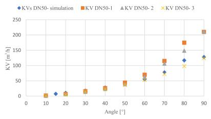
FIG. 3. Examples of the flow rate coefficient for butterfly valves from different manufacturers against computational data.
