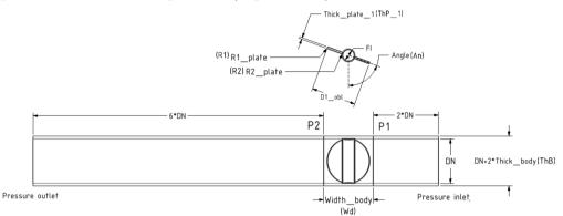
FIG. 1. Dimensions of the butterfly valve.
