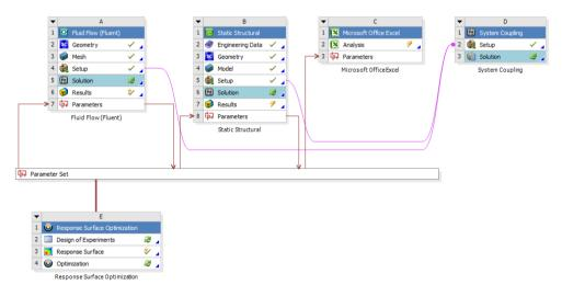
FIG. 4. The multi-objective optimization procedure.
