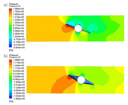
FIG. 5. Pressure contour for valve dimensions: a) ThP\_2\_2 = 1 mm, R1 = 0.1 mm, R2 = 0.1 mm at the middle plane and 70 degree opening, b) ThP\_2\_2 = 6 mm, R1 = 0.55 mm, R2 = 22.55 mm.
