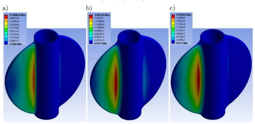
FIG. 10. Equivalent von Mises stress for optimal candidates: a) full second-order polynomials, b) non-parametric regression, c) Kriging.
