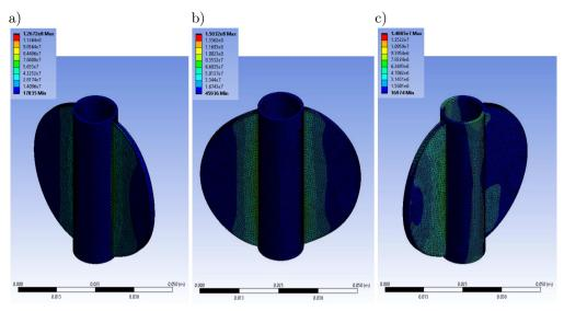
FIG. 9. Equivalent von Mises stress for initial disc geometry and opening angle: a)  $10^{\circ}$ , b)  $50^{\circ}$ , c)  $80^{\circ}$ .
