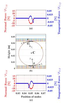
FIG. 15. Normal and frictional force distribution at t = 5 s during the anticlockwise rolling of the grasped disc.
