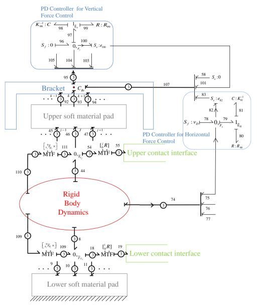
FIG. 9. Schematic diagram showing interconnected subsystems of the system considered for the soft contact manipulation.
