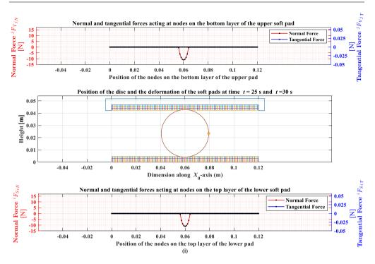
FIG. 16. The positions of the disc and the distribution of contact forces along with the deformation in layers of the soft pads at various instants of time: a) t = 0.375 s, b) t = 2.5 s, c) t = 5 s, d) t = 7.5 s, e) t = 10 s and t = 15 s, f) t = 17.5 s, g) t = 20 s, h) t = 22.5 s, i) t = 25 s and t = 30 s.
