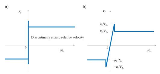
FIG. 6. a) Classical Coulomb's friction model, b) proposed friction model using momentary spring-dashpot in Kelvin–Voigt configuration.
