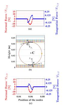
FIG. 14. Normal and frictional force distribution at t = 0.125 s during the grasping of the disc.
