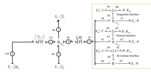
FIG. 5. The bond graph model for the upper contact interface.
