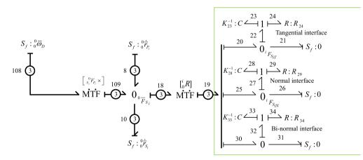
FIG. 4. The bond graph model for the lower contact interface.
