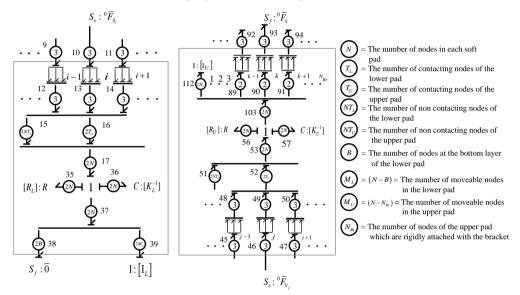
FIG. 7. The bond graph model for lower and upper soft material pads.
