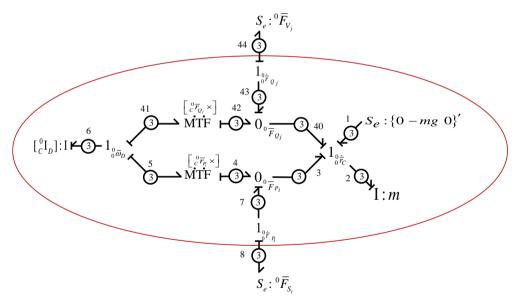
FIG. 3. The bond graph model for rigid body dynamics subjected to contact forces at lower and upper contact interfaces.
