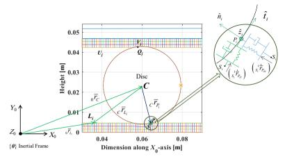
FIG. 2. Contact detection and modeling of the contact interfaces between the rigid object and the soft material pads.
