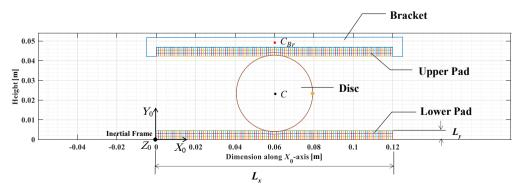
FIG. 1. The system considered for the soft contact manipulation of a rigid object.
