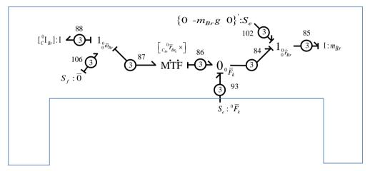
FIG. 8. The bond graph model for the rigid bracket connected rigidly with nodes on the upper layer of the upper soft pads.
