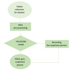
FIG. 2. The proposed system flow diagram.
