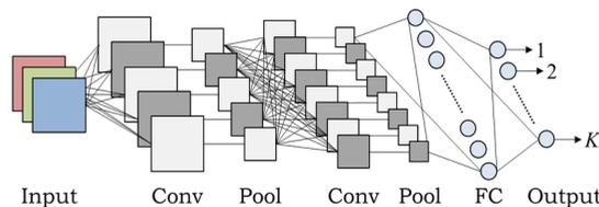
FIG. 6. CNN architecture.
