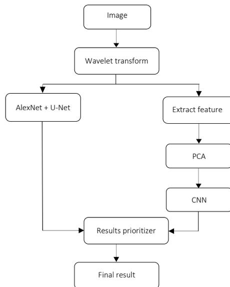
FIG. 4. Proposed architecture model.
