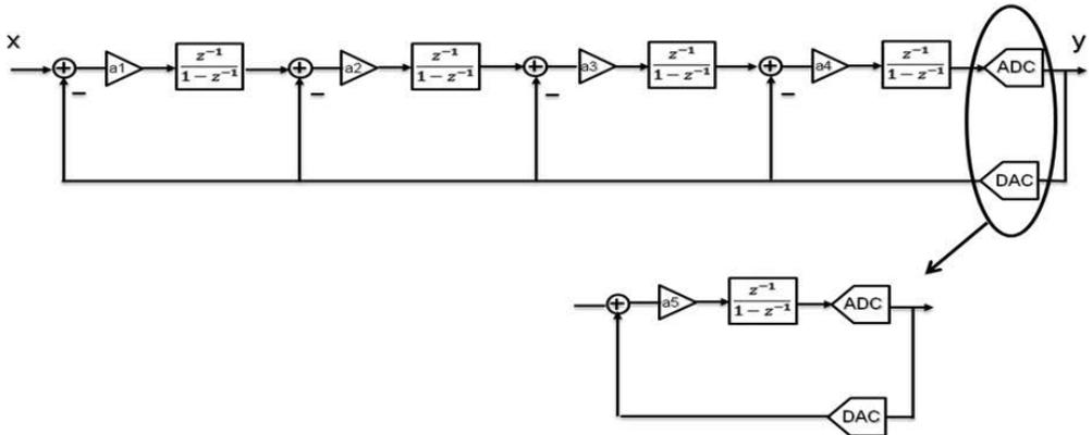
FIG. 4. Block diagram of fifth order single loop SDM.
