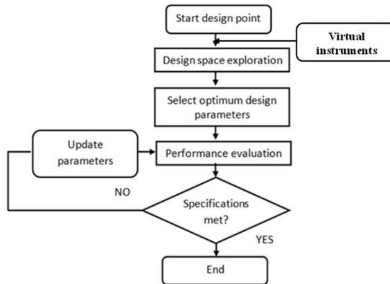
FIG. 3. Proposed design methodology flowchart.
