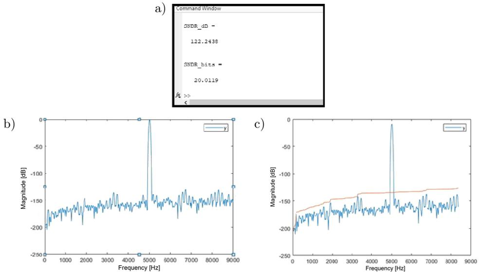
FIG. 7. a) SNDR computed, b) signal spectrum, c) integrated noise power.
