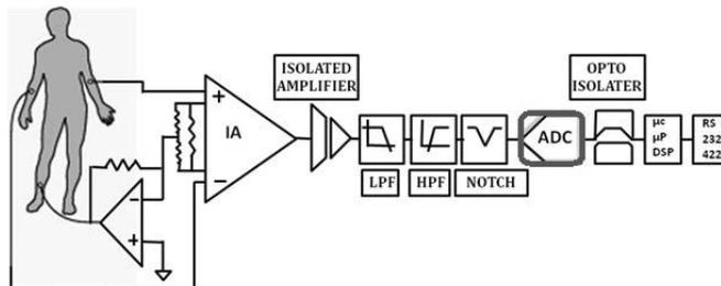
FIG. 2. ECG signal processing system.
