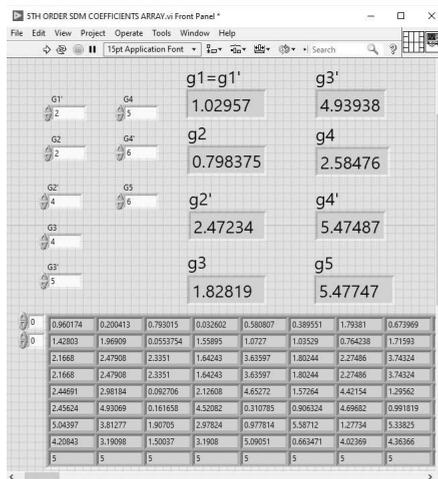
FIG. 6. Front panel of virtual instrument displaying integrator scaling.
