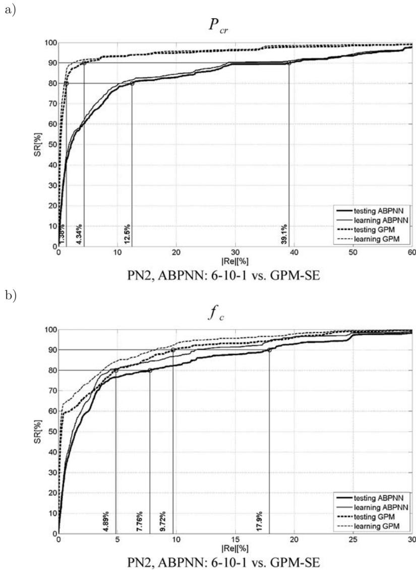
**Fig. 3.** Comparison of Success Ratios for data set PN2 applying ABPNN and GPM for prediction  $P_{cr}$  and identification  $f_c$ .
