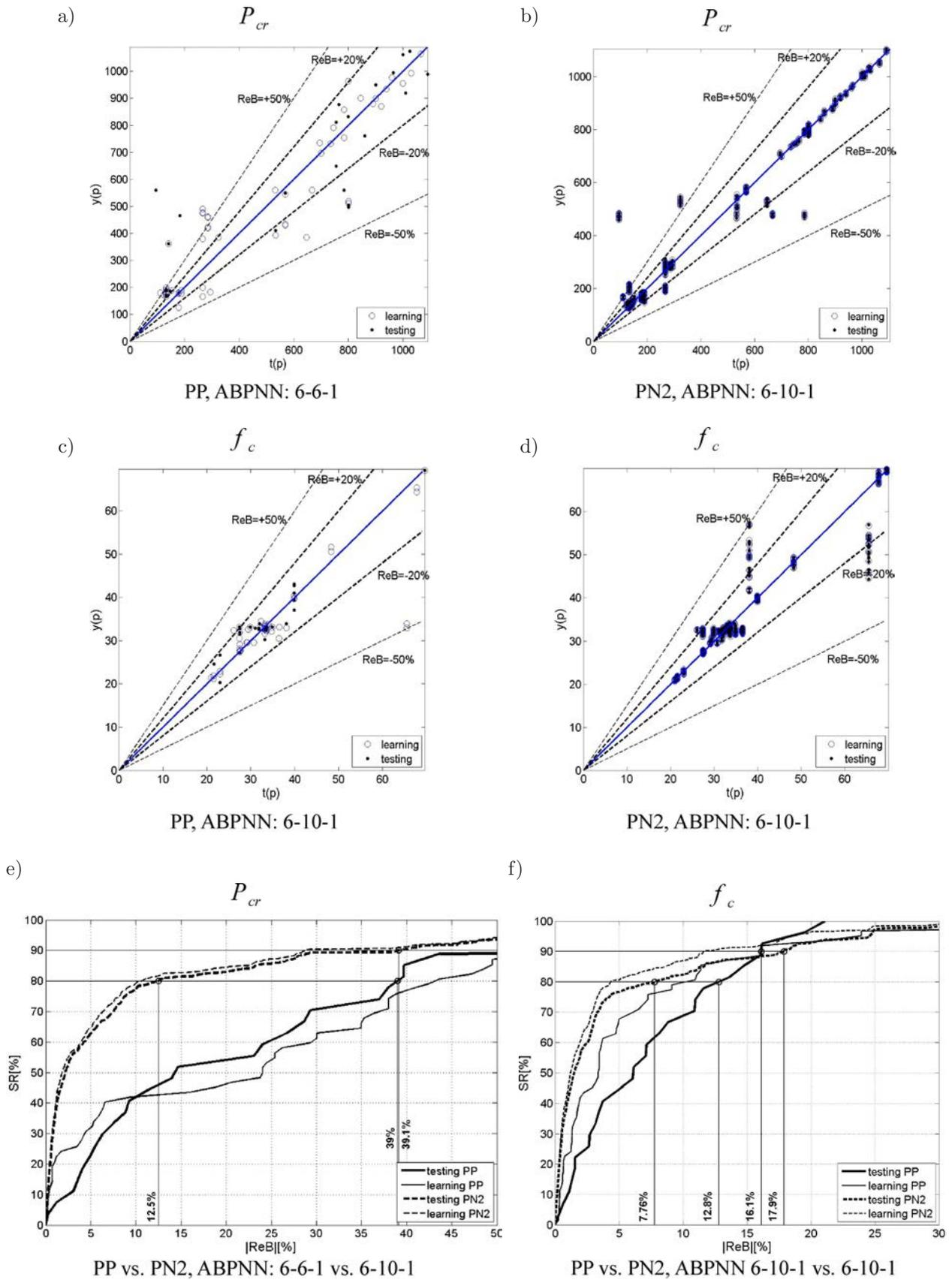
**Fig. 1.** a, b, c, d) Bound errors for application of ABPNN for prediction  $P_{cr}$  and identifying  $f_c$  input pattern sets computed for primary and noisy patterns PP and PN2; e, f) Comparison of Success Ratio Curves for data sets PP vs. PN2.
