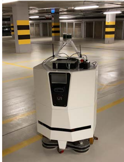
FIG. 1. Photo of a prototype of the cleaning robot being developed by our industrial partner, the United Robots company. The robot is equipped with sensors such as LIDARs and RGBD cameras, which ensure that all safety measures are taken into account, and the accurate position in the global frame is known. The photo is for illustrative purposes only, and the details regarding robot control and navigation are outside of the scope of this work.
