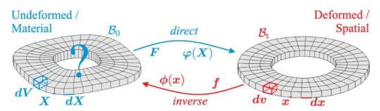
Fig. 1. Inverse form finding: the material configuration  $\mathcal{B}_0$  is sought while the desired spatial configuration  $\mathcal{B}_t$  is given; illustration of the direct (blue) and inverse (red) mechanical formulation.
