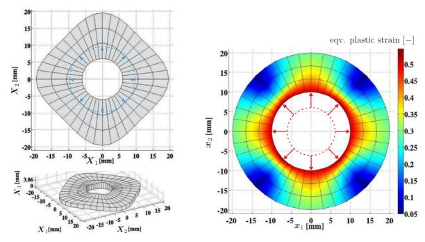
Fig. 4. Example 1: the found optimal material configuration ( $X_{\text{Opt}} = X_{\text{current}}$ ) of the workpiece (left). The target spatial configuration of the workpiece ( $x_{\text{current}} = x_{\text{target}}$ ) after the final direct simulation based on the determined optimal material configuration (right).
