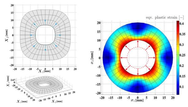
Fig. 5. Example 2: the found optimal material configuration ( $X_{\text{Opt}} = X_{\text{current}}$ ) of the workpiece (left). The target spatial configuration of the workpiece ( $x_{\text{current}} = x_{\text{target}}$ ) after the final direct simulation based on the determined optimal material configuration (right).
