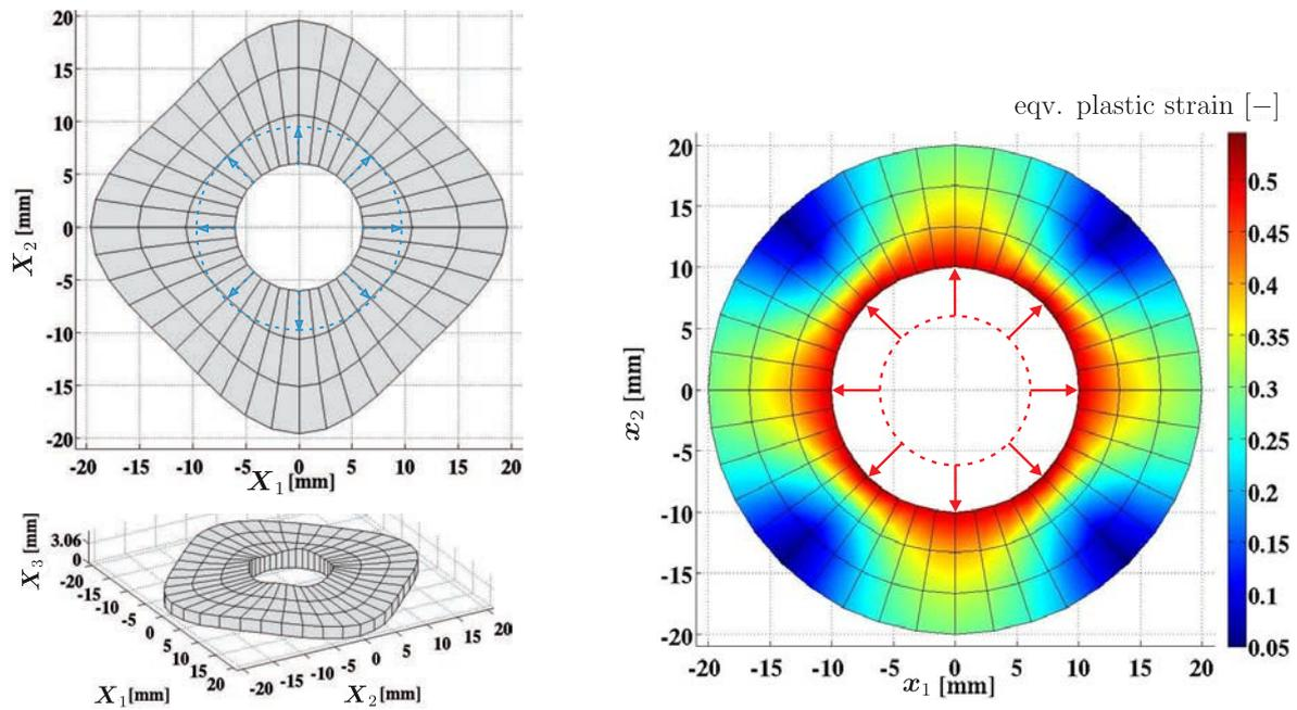
**Fig. 4. Example 1:** the found optimal material configuration ( $\mathbf{X}_{\text{Opt}} = \mathbf{X}_{\text{current}}$ ) of the workpiece (left). The target spatial configuration of the workpiece ( $\mathbf{x}_{\text{current}} = \mathbf{x}_{\text{target}}$ ) after the final direct simulation based on the determined optimal material configuration (right).
