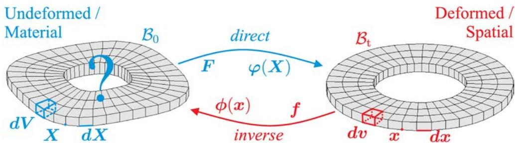
**Fig. 1.** Inverse form finding: the material configuration  $B_0$  is sought while the desired spatial configuration  $B_t$  is given; illustration of the direct (blue) and inverse (red) mechanical formulation.
