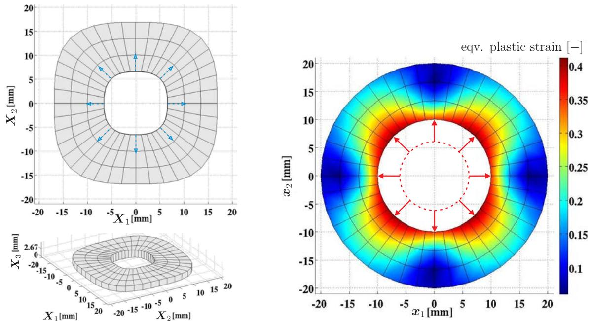
**Fig. 5. Example 2:** the found optimal material configuration ( $\mathbf{X}_{\text{Opt}} = \mathbf{X}_{\text{current}}$ ) of the workpiece (left). The target spatial configuration of the workpiece ( $\mathbf{x}_{\text{current}} = \mathbf{x}_{\text{target}}$ ) after the final direct simulation based on the determined optimal material configuration (right).
