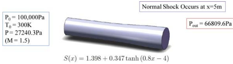
Fig. 17. Normal shock nozzle geometry.
