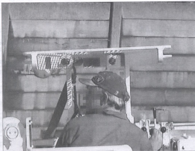
Fig. 1. Falling-object protective structures mounted on the self-propelled mining machine frame
