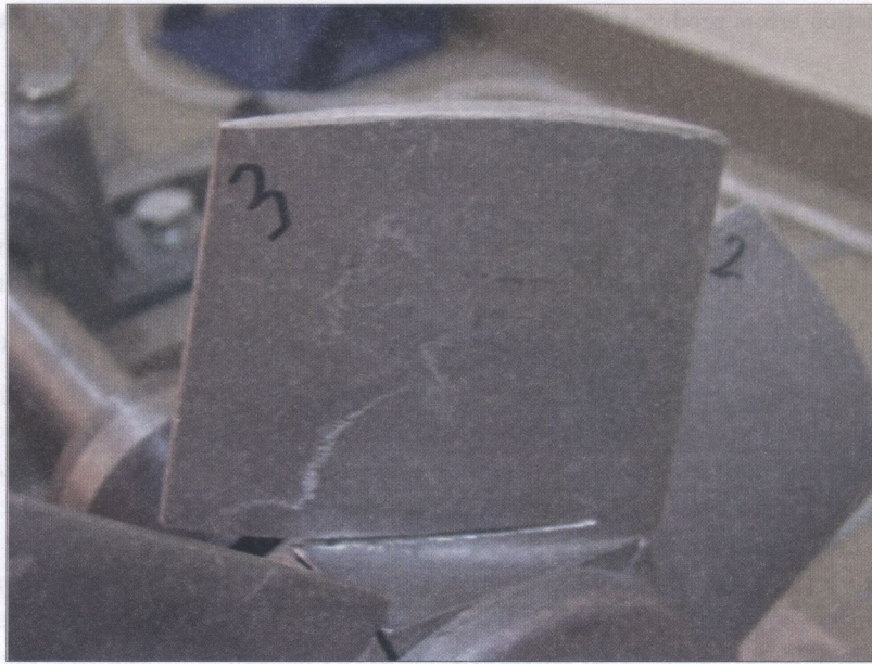
Fig. 7. Simulation of crack at blade
