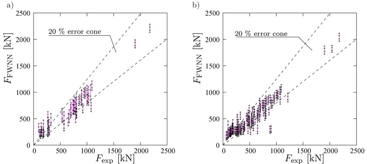
**Fig. 6.** Cases **A** a) and **E** b). Comparison of experimental data  $F_{exp}$  and FWNN results  $F_{FWNN}$  for the  $\alpha$ -cuts for  $\alpha = 0.9, 0.75$ .
