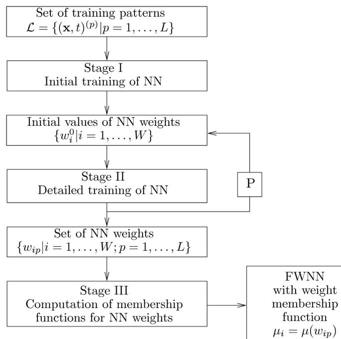
Fig. 1. Schematic algorithm for a Fuzzy Weight Neural Network (FWNN) formulation.
