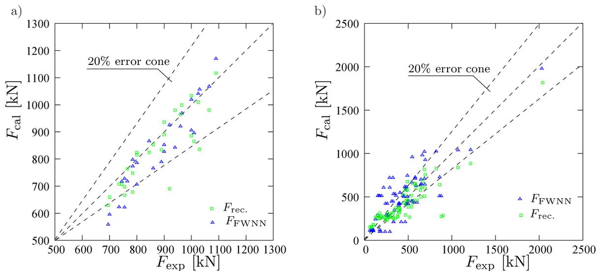
**Fig. 7.** Comparison of both the critical load calculated according to design recommendation [5] and calculated by FWNN for  $\alpha$ -cross-section 1.0 against the experimental results from a) Chudyba's database, b) Cranston's database.
