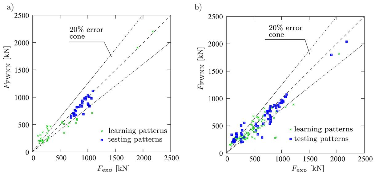
**Fig. 3.** Comparison of NN simulation results versus experimental data for: a) case **A**, b) case **E**.
