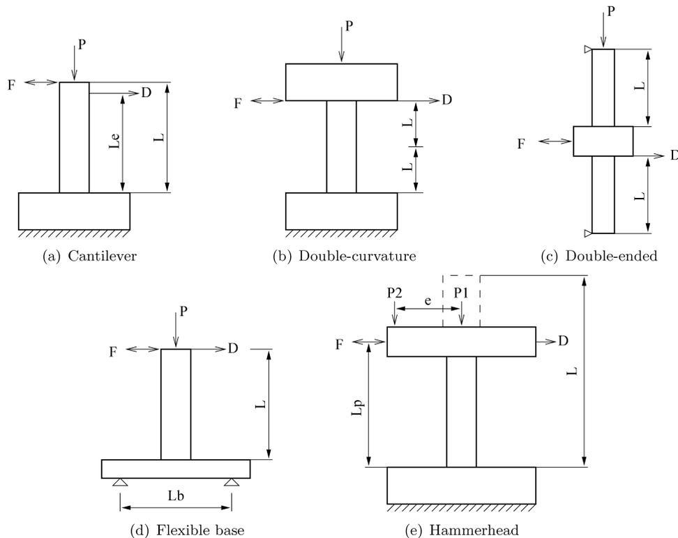
**Fig. 2.** Column test configuration in PEER database.
