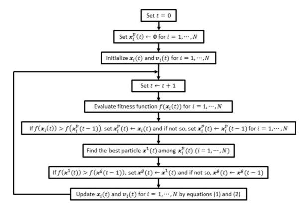
Fig. 1. Flowchart of original PSO algorithm.
