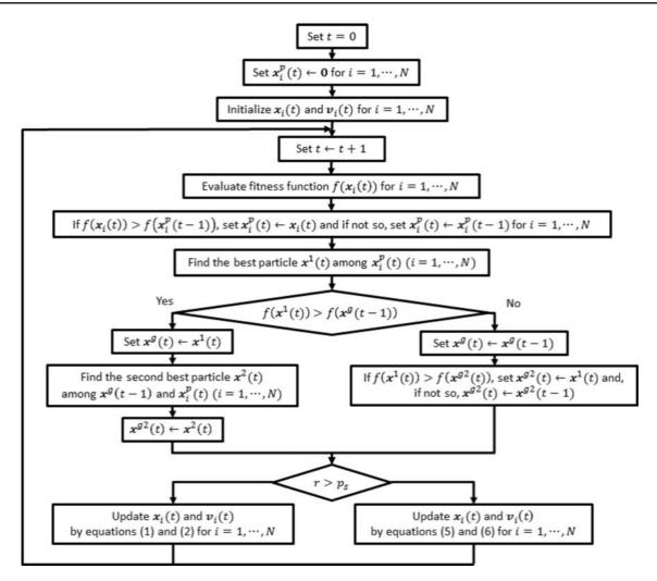
Fig. 2. Flowchart of improved PSO algorithm.
