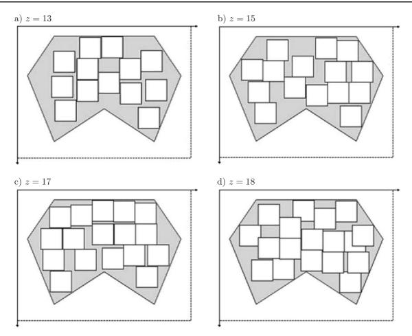
Fig. 9. Best item placement determined by improved PSO in case B.  $\,$
