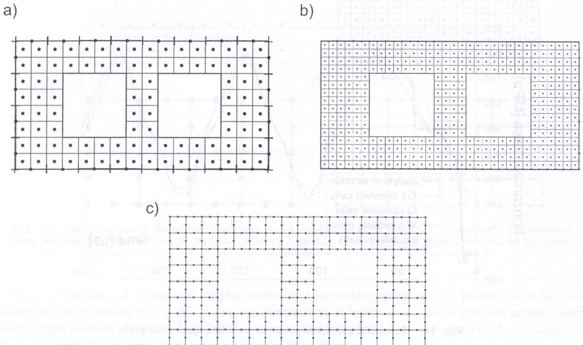
Fig. 18. Discretization of the plate with square holes; a) 96 constant cells, 40 boundary elements, b) 384 constant cells, 80 boundary elements, c) 96 quadratic cells, 40 boundary elements
