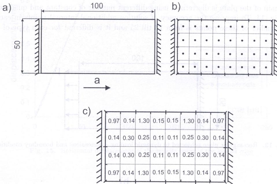
Fig. 11. Rectangular plate subjected to the inertial loading; a) dimensions and boundary conditions, b) discretization, c) percentage stress error in each cell
