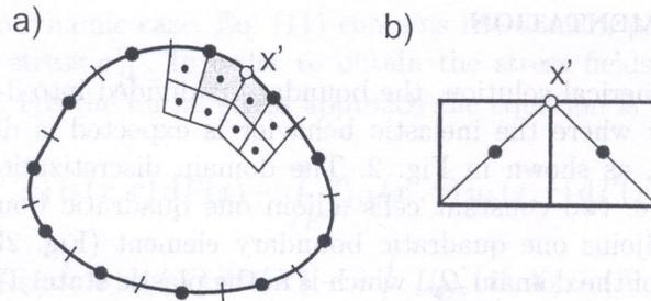
Fig. 3. Boundary collocation point – constant cells; a) singular cells at the collocation point, b) division of cells into triangles
