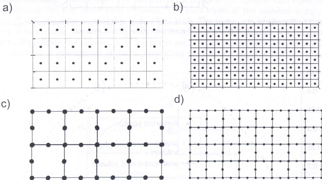
Fig. 14. Discretization of the rectangular plate; a) 32 constant cells, 12 boundary elements, b) 128 constant cells, 24 boundary elements, c) 8 quadratic cells, 12 boundary elements, d) 32 quadratic cells, 24 boundary elements
