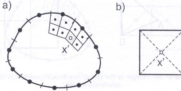
Fig. 6. Internal collocation point – constant cells; a) singular cell at the collocation point, b) division of the cell into triangles
