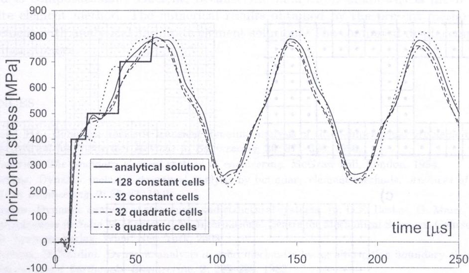
Fig. 16. Horizontal normal stress at the middle point of the plate
