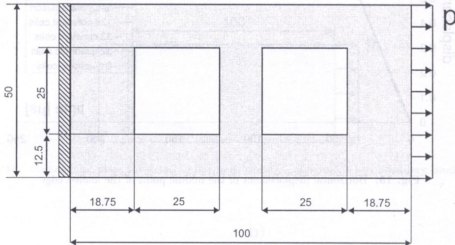
Fig. 17. Plate with square holes subjected to dynamic loading – dimensions and boundary conditions
