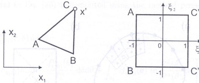
Fig. 5. Transformation of the triangle in the global coordinate system into the square in the local coordinate system
