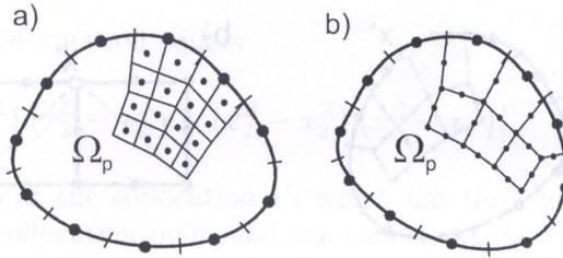
Fig. 2. Discretization of the body; a) constant cells, b) quadratic cells
