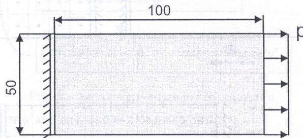
Fig. 13. Rectangular plate subjected to dynamic loading – dimensions and boundary conditions
