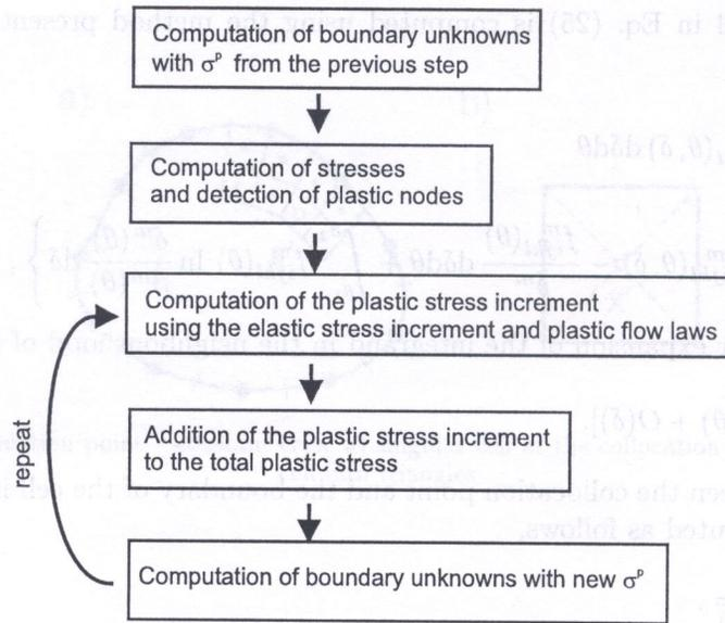
Fig. 9. Iterative procedure in each time step
