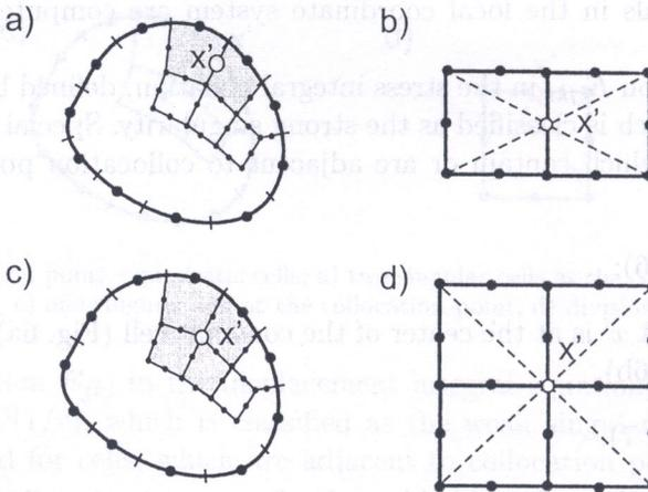
Fig. 7. Internal collocation point – quadratic cells; a) two singular cells at the collocation point, b) division of two cells into triangles, c) four singular cells at the collocation point, d) division of four cells into triangles
