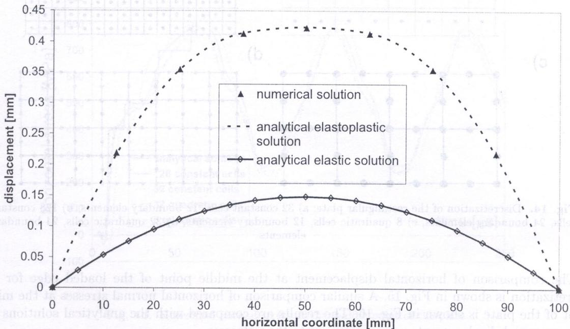
Fig. 12. Displacements of the upper edge of the plate
