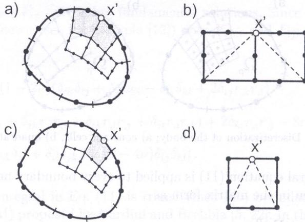
Fig. 4. Boundary collocation point – quadratic cells; a) two singular cells at the collocation point, b) division of two cells into triangles, c) one singular cell at the collocation point, d) division of one cell into triangles
