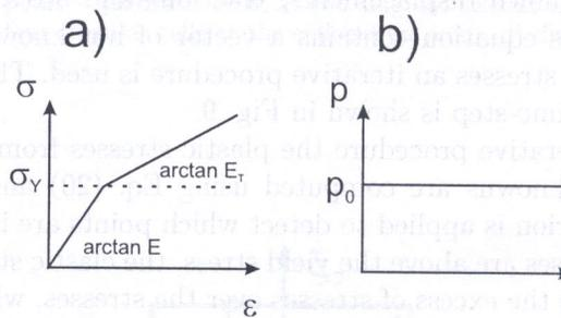
Fig. 10. a) stress–strain relation b) time history of loading
