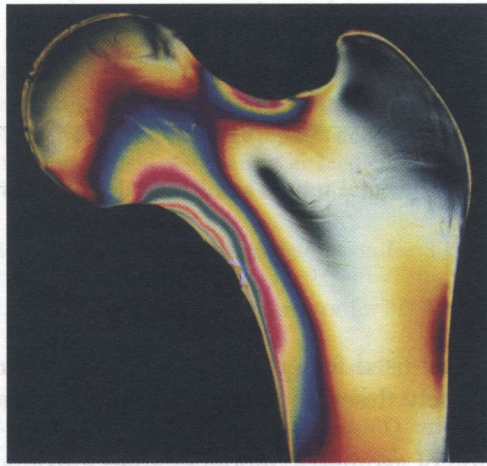
Fig. 18. Picture of photo-elastic image of the bone's longitudinal cross-section
