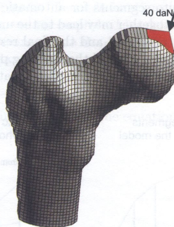
Fig. 16. A view of numerical model of the femoral head (note the marked way of load application according to Pauwels' diagram – grid every 1 mm)
