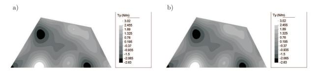
Fig. 12. Predicted in-plane stress resultant  $t_y$  at 11.5 kHz: a) WBM T2 (192 dofs), b) FEM (349,173 dofs).
