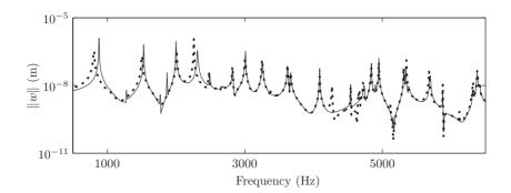
**Fig. 29.** Frequency response function for response point  $w_1$  (dashed: WBM; solid: WBM *CF*).
