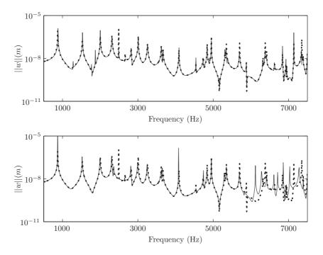
Fig. 25. Frequency response function for response point  $w_1$  (dashed: FE reference 121,503dofs; solid: WBM *CF T1* (top) or FEM 19,833 dofs – 7elements/ $\lambda_t$  (bottom)). The WBM *CF T1* and FEM of 19,833 dofs have a comparable computational load.
