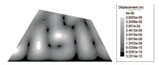
Fig. 9. Amplitude of the forced displacement at 11.5 kHz predicted by the WBM T2.
