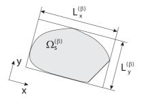
Fig. 6. Definition of the bounding box for subdomain  $\beta$ .
