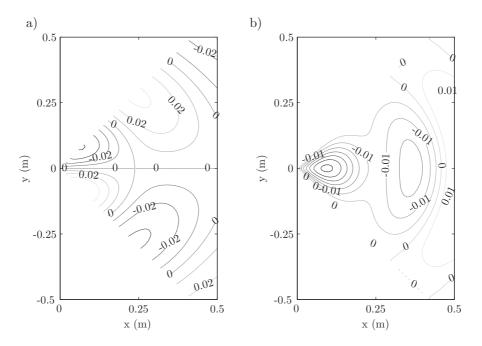
Fig. 3. Displacement field corresponding to the anti-symmetric dilatational and symmetric rotational eigenfunctions with  $\lambda_l^* = \lambda_t = 1.8$  for a simply supported infinite wedge with  $\alpha = 100^\circ$ ,  $k_l = 12.0$  m<sup>-1</sup> and  $k_t = 20.2$  m<sup>-1</sup>: a) radial displacement  $w_r$ , b) angular displacement  $w_{\theta}$ .
