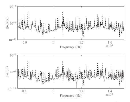
Fig. 26. Frequency response function for response point  $w_1$  in the mid-frequency range (dashed: FE reference 121,503dofs; solid: WBM *CF* 11 (top) or FEM 19,833 dofs – 7elements/ $\lambda_t$  (bottom)). The WBM *CF* 11 and FEM of 19,833 dofs have a comparable computational load.
