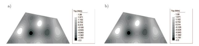
Fig. 13. Predicted in-plane stress resultant  $t_{xy}$  at 11.5 kHz: a) WBM T2 (192 dofs), b) FEM (349,173 dofs).
