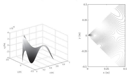
Fig. 4. Radial stress field corresponding to the anti-symmetric dilatational and symmetric rotational eigenfunctions with  $\lambda_l^* = \lambda_t = 1.8$  for a simply supported infinite wedge with  $\alpha = 100^\circ$ ,  $k_l = 12.0 \text{ m}^{-1}$  and  $k_t = 20.2 \text{ m}^{-1}$ .
