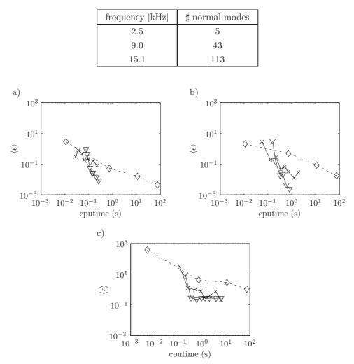
**Fig. 24.** Comparison of the convergence of the FEM  $(-\diamond -)$ , the WBM  $(-\times -)$  and the WBM *CF*  $(-\nabla -)$ : a) 2.5 kHz, b) 9 kHz, c) 15.1 kHz.
