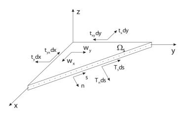
Fig. 1. In-plane forces acting on a plate section.
