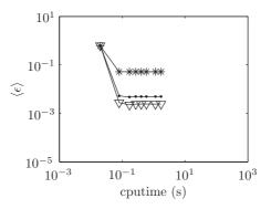
Fig. 15. Influence of the FE reference model on the convergence of the WBM at 17.2 kHz: FE reference of 366,900 dofs (-\*-), 1,458,906 dofs  $(-\cdot-)$ , 2,977,089 dofs  $(-\nabla-)$ .
