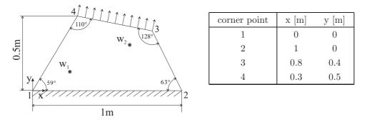
Fig. 8. Geometry of a convex problem without singularities.
