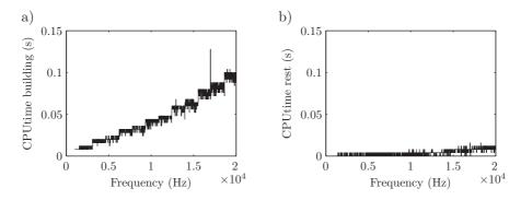
Fig. 18. Frequency dependent computation time for the WBM with T = 1: a) cpu time for model construction, b) cpu time for remaining tasks.
