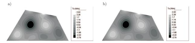
Fig. 11. Predicted in-plane stress resultant  $t_x$  at 11.5 kHz: a) WBM T2 (192 dofs), b) FEM (349,173 dofs).
