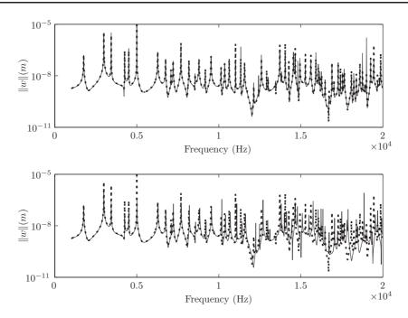
Fig. 16. Frequency response function for response point  $w_1$  (dashed: FE reference 366,900 dofs; solid: WBM T1 (top) or FEM 3,774 dofs – 4elements/ $\lambda_b$  (bottom)). The WBM T1 and FEM of 3,774 dofs have a comparable computational load.
