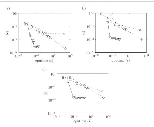
Fig. 14. Comparison of the convergence of the FEM with quadrilateral  $(-\diamond -)$  and triangular  $(-\times -)$  discretisations and the WBM  $(-\nabla -)$ : a) 6 kHz, b) 11.5 kHz, c) 17.2 kHz.
