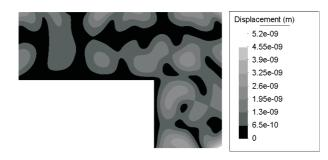
Fig. 20. Amplitude of the forced displacement at 9 kHz predicted by the WBM CF T2.
